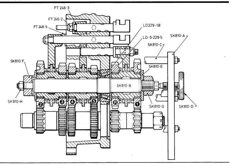
For this operation we recommend the use of a Hewland fork setting jig assembly (SK 810). This is also designed for fork setting & assembly operations on LD 4-speed gear boxes and comprises the following components:-
