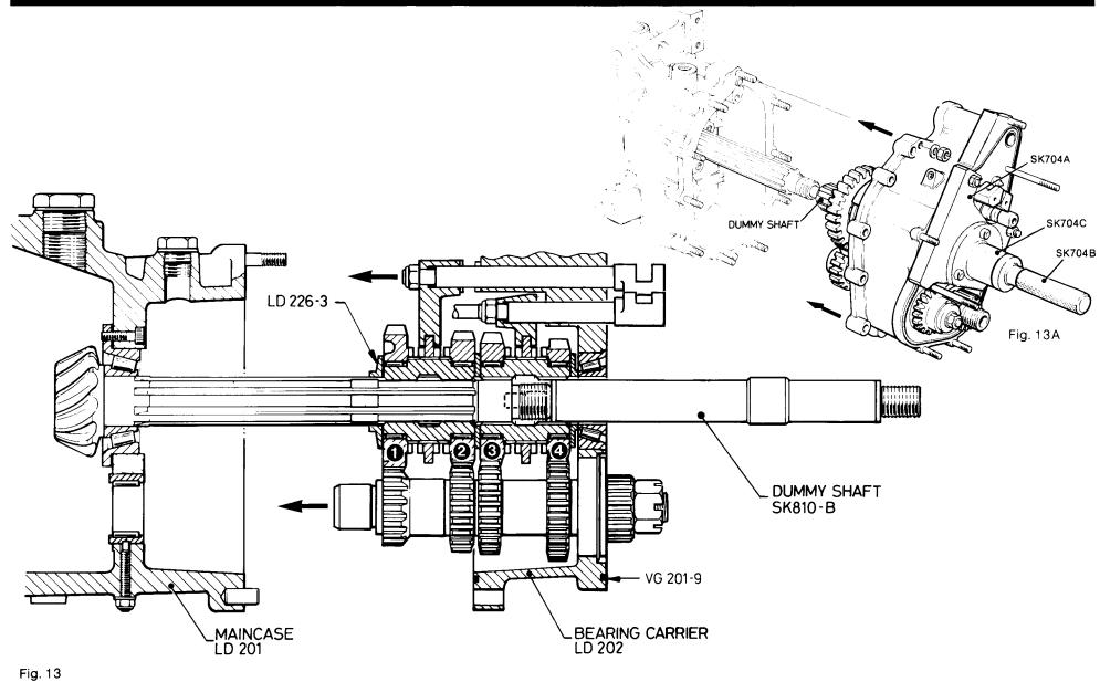
LD 4-speed gearboxes can be assembled using either the earlier type of dummy shaft or the later type, which is also used for 5-speed gearboxes. The procedure is the same in both cases.
