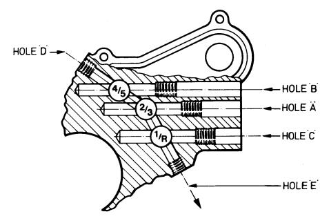
Positioning mark on collar of 1st/rev selector rod must face in direction of this arrow.
